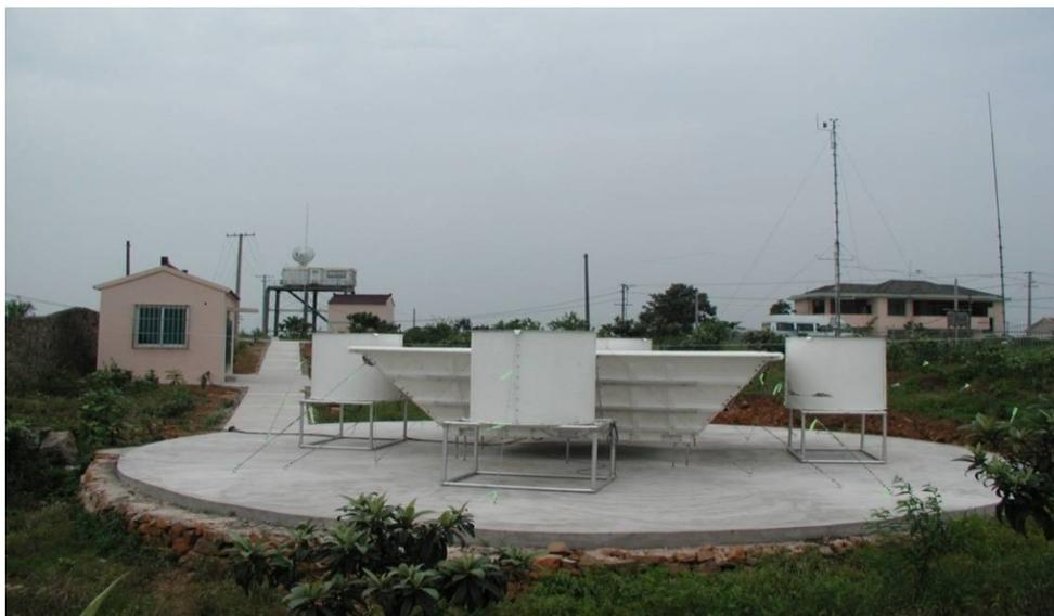
Fig.1: Wind Profiler Radar (WPR) installed at Dongshan (31°4'47" N; 120°26'3" E), China
